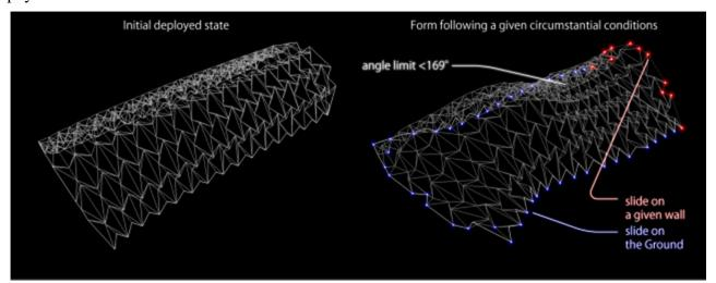
Figure 7: Geometric Constraints.
