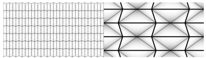
Figure 1: Left: A variational waterbomb corrugation pattern. Right: close-up of the pattern (thick: mountain fold, thin: valley fold). A vertex with 4 (or 2) mountain folds is convex (or concave resp.).
