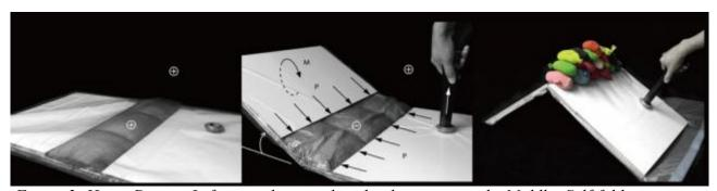
Figure 3: Hinge Design. Left: particles are placed in between panels. Middle: Self-folding moment is induced by the vacuum. Right: The vacuum keeps the hinge stiff.
